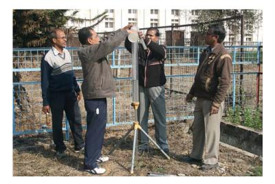
Determination of saturated hydraulic conductivity using Guelph Permeater
